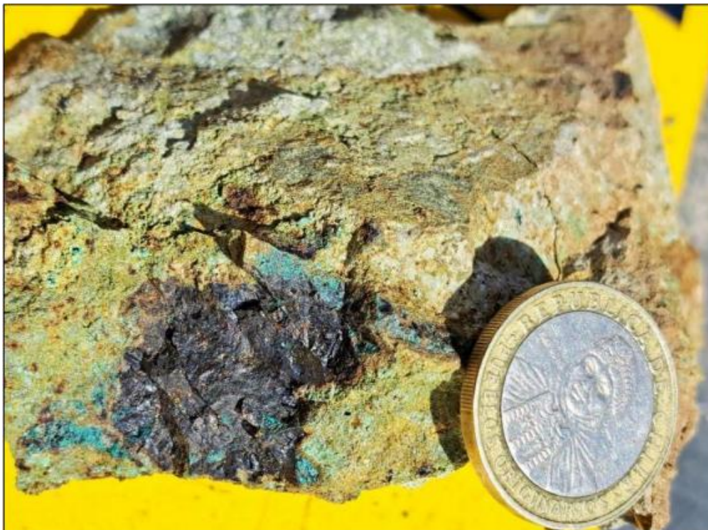
Figure 2 – Significant copper (malachite, bornite and chalcopyrite) mapped in outcrop, sample number CPO0008615, returned 5.37% Cu. (ASX Announcement 21 November 2023)
