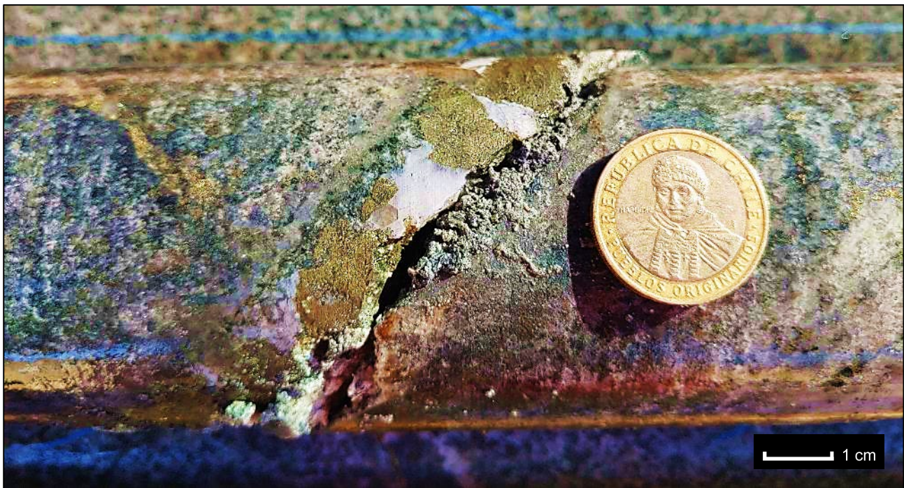
Figure 3: Course grained Chalcopyrite mineralisation logged in CMLCD011 (381m) (Refer Appendix E).
