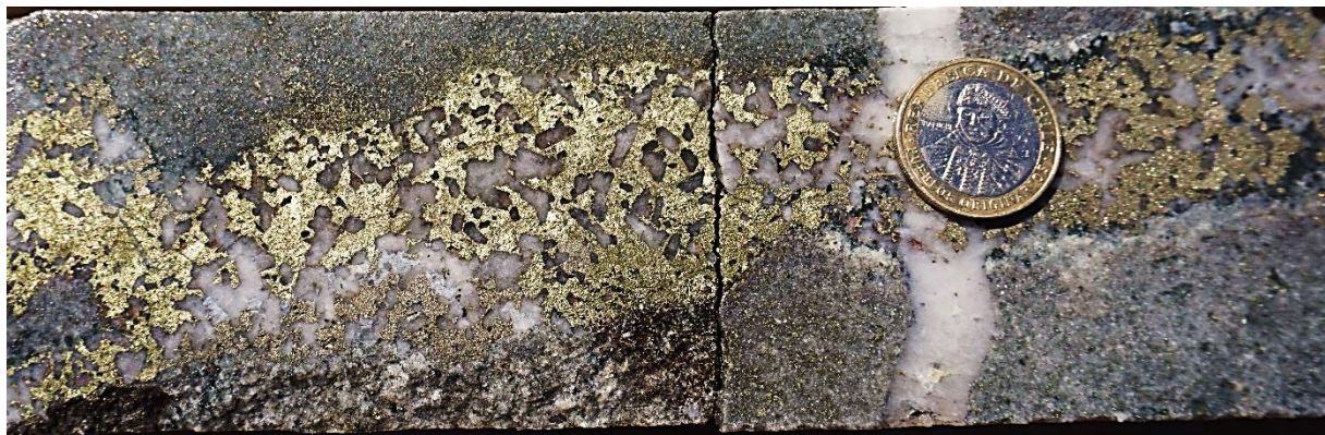
Figure 1: High-grade near surface Cu mineralisation, CMLCD005A, 1m @ 4.01% Cu (131 – 132m).
