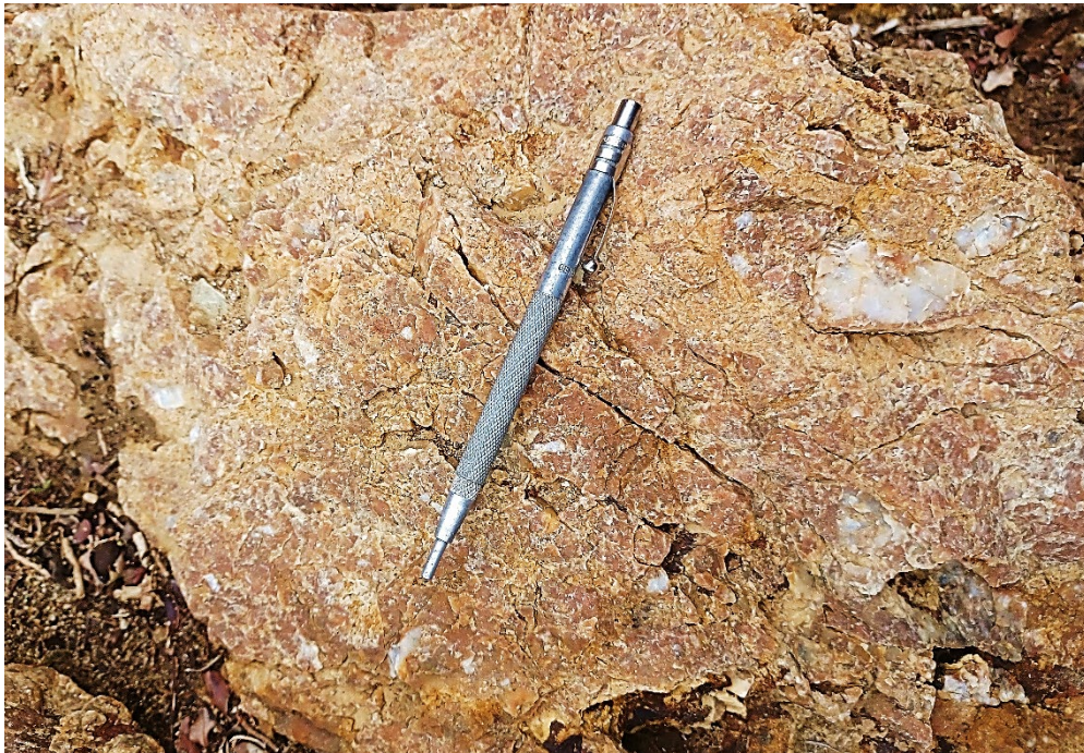
Figure 4: Silicified breccias identified at the T4 target area.
